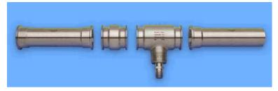
To achieve optimum performance of the Sanitary Turbine Flowmeter, a minimum of 10 pipe diameters upstream and 5 pipe diameters downstream of meter size pipe must be used.
