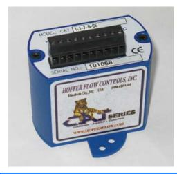
The CAT1 is a microprocessor controlled 2-wire 4-20mA transmitter. The CAT1 converts a low level, frequency signal from a flowmeter sensor into an analog 4-20mA output. The output is proportional to the flow rate.
