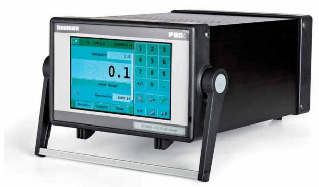
The Beamex® POC6 can be used as a stand-alone pressure controller or together with Beamex® MC5 and MC5P Calibrators.
